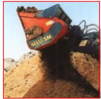
ALLU is the easy way to make different soil mixtures
