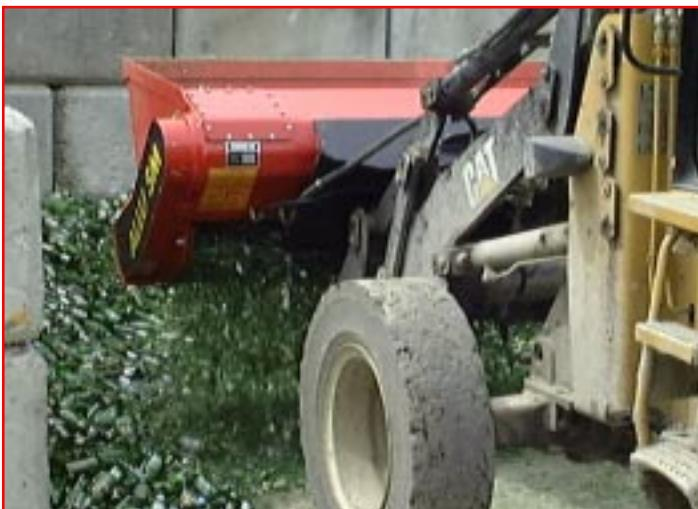
ALLU buckets are excellent for processing materials like glass bottles. Above an ALLU SM2-23 attached to a Cat IT14
