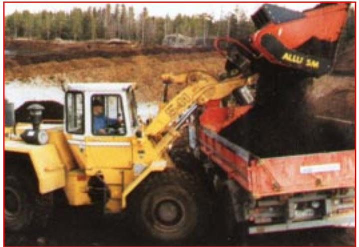
ALLU SM 4-23. Material flows smoothly through the ALLU SM due to carefully designed frame and size of screening area, which is large in proportion to bucket volume.
