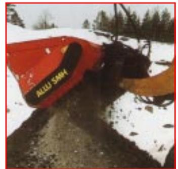
Crush lightweight concrete
